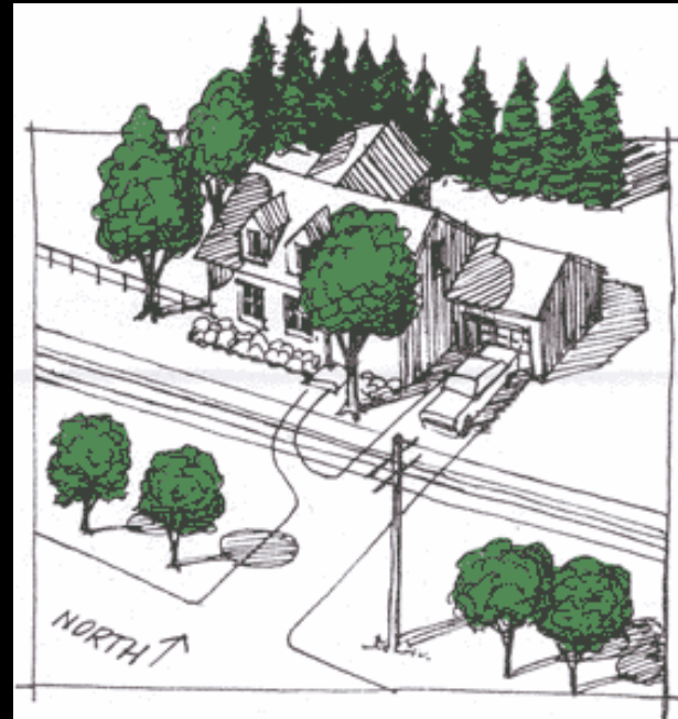
Right Short flowering trees don't clash with overhead utility lines. Large deciduous trees on the southeast, southwest, and west provide cooling shade in summer, and don't obstruct the low winter sun. An evergreen windbreak on the north blocks cold winter winds.
